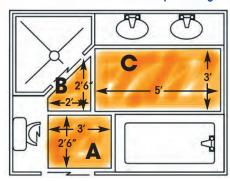
Colored shaded areas represent where you would install your Cable System. **A** is 2'6" x 3' = 7.5 ft² (0.76 m x 0.91 m = 0.69 m²) **B** is (2'6" x 2')  $\div$  2 = 2.5 ft² ([0.76 m x 0.61 m]  $\div$  2 = 0.23 m²) **C** is 3' x 5' = 15 ft² (0.91 m x 1.52 m = 1.39 m²)
